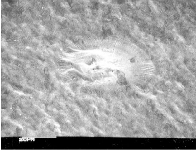
Fig. 10 Backside of a 6 micrometer thick aluminum foil struck with an EV and a deposit of aluminum oxide
